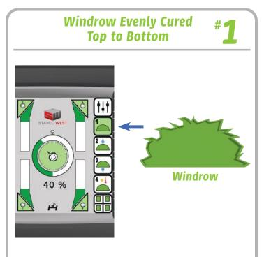
When a windrow is evenly cured, use Steam Preset #1, and start with the steam rate at 40%. Adjust steam rate as needed.
