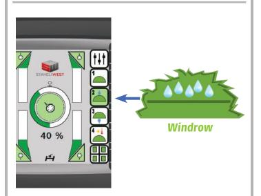
When a windrow has more moisture on top than on bottom, use Steam Preset #2, and start with the steam rate at 40%. Adjust steam rate as needed.
