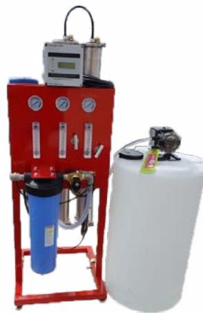
Reverse Osmosis (RO) Unit
