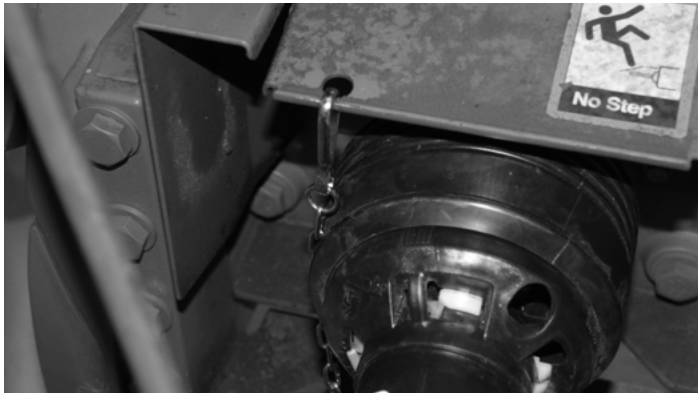
Secure anti-rotating shield clip as shown.
